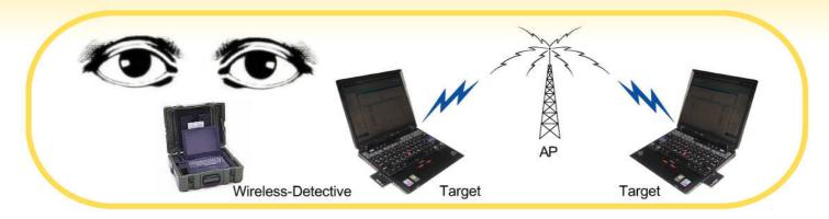
Different with normal Sniffer, it can record session then decode and recombine packets to reproduce the original file. If there's common WEP key encrypted wireless transmission, Wireless-Detective can offer WEP decryption function for you. Wireless-Detective can decrypt the WEP key of the length of 64, 128, 256 bits or the special defined WEP key and can also decrypt part of WPA encryption.
